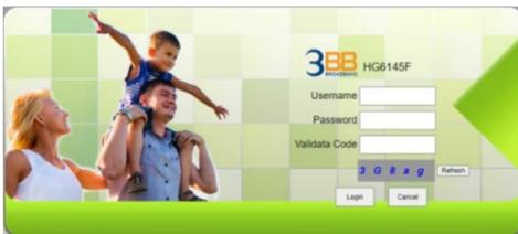
After login in to the GPON Terminal (HG6145F), you will see the following interface. You can check, configure and modify all the settings.
